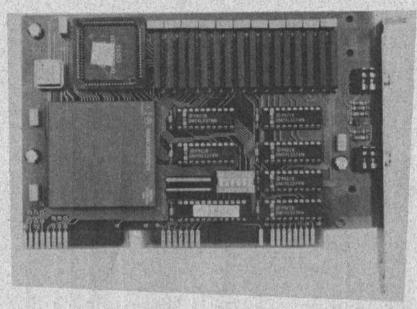
The QXL turns the common PC into a QL compatible. The package comprises a half card that plugs into an 8 or 16 bit standard ISA slot and a diskette loaded with a QDOS compatible operating system and a SuperBasic compatible interpreter. After installation simply type QXL and the PC will appear to be a QL allowing QL programs to be run from QL format diskettes.
