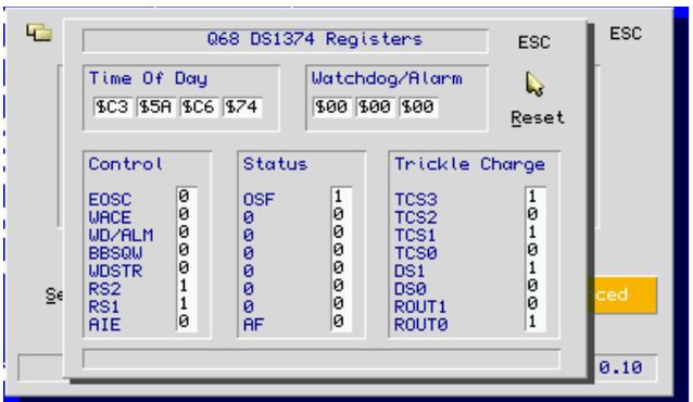
Note that the Time Of Day values are displayed with the least significant byte first, and the most significant byte last. Clicking on Reset will reset the Time Of Day and Watchdog/Alarm registers to zero, and the Control, Status, and Trickle Charge registers to values suitable for the Q68.
